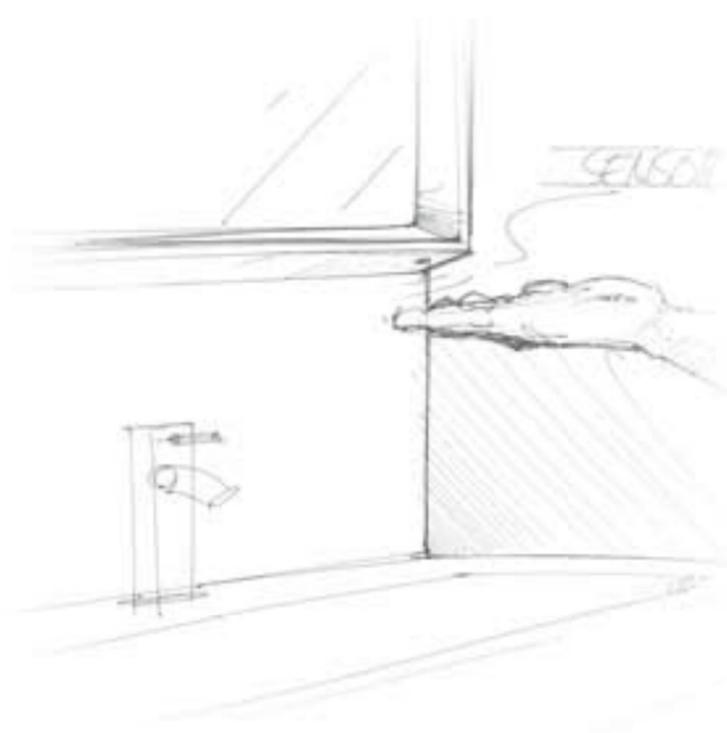
**SENSOR-CONTROLLED MIRROR LIGHT** An integrated sensor ensures that the mirror lighting with dimmer function can be activated without any contact at all. This is not only more hygienic, but also highly practical, for instance with wet hands. It is available for 2nd floor, Darting New, Delos, DuraStyle, Fogo, Happy D.2, Ketho, Starck and Vero, and recently L-Cube and Cape Cod as well.
